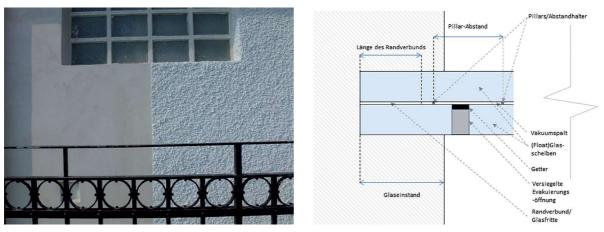
Fig. 6: Aerogel-plaster test surfaces (Image by the Author), fig. 7: Schematic Constituents of vacuum glazing products (Image by the Author)
