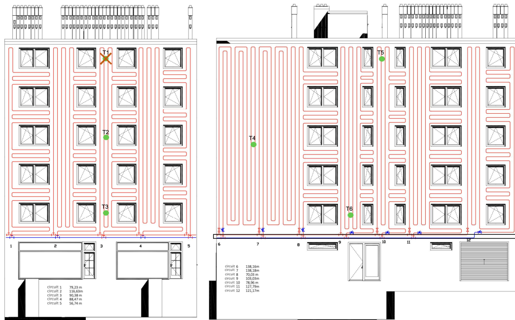
Fig. 3: Position of the façade core temperature sensors (T2-T6, green dots) on the façade in Rittergasse (left) and GroßeNeugasse (right). T1 had to be disconnected to allow the installation of the heating water flow supervision system. The red lines show the heating circuit piping.
