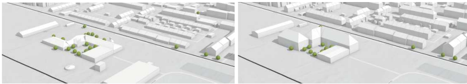
1: Building models derived from OpenStreetMap, 2: Level of detail 2 buildings from OpenData BY
