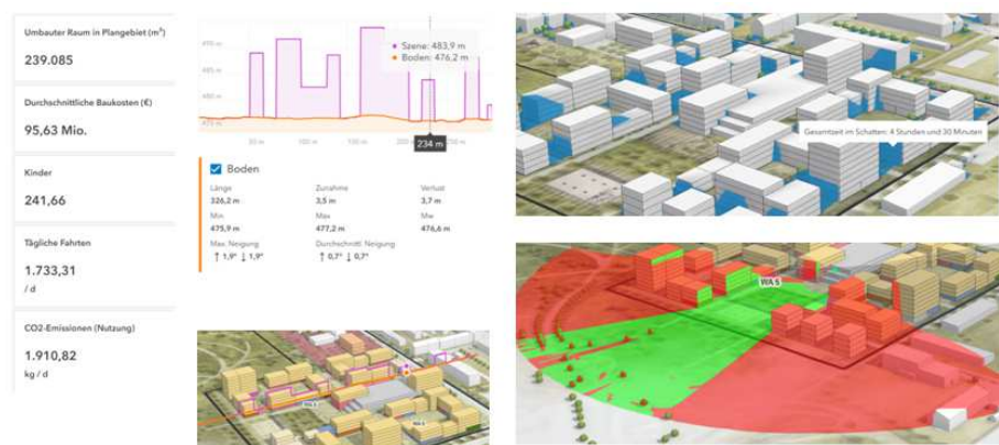
8: Indicators on size, cost, demography, mobility and emissions, 9: Selected shading and viewshed analyses.
