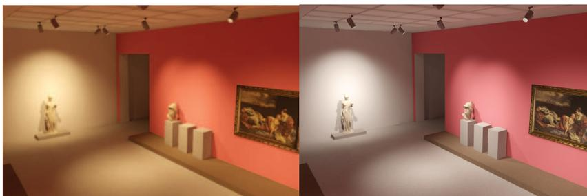
Fig. 1: Color temperature comparison. Left: warm white (3000K). Right: cool white (5000K)
