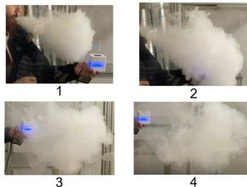
Fig. 10: Experiments in a closed room with e-cigarette: distribution of the cloud in the room.
