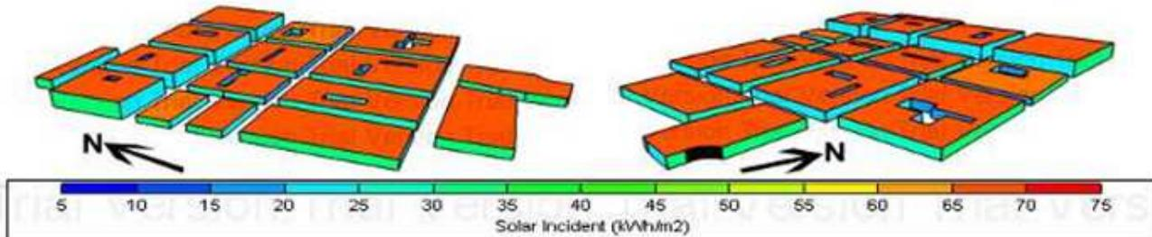
Fig.13: Solar Incident (KWh/m2) in Summer. Left: Show South, West façades, Right: Show North, East façades
