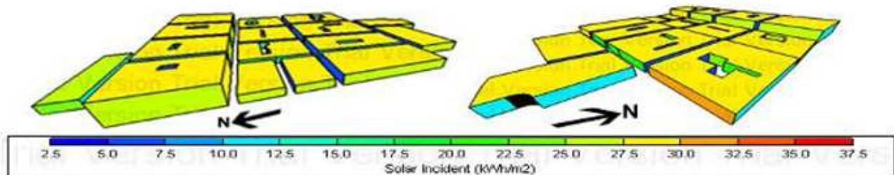
Fig. 10: Solar Incident (Kw/m<sup>2</sup>) in Winter. Left: Show South, West façades, Right: Show North, East façades
