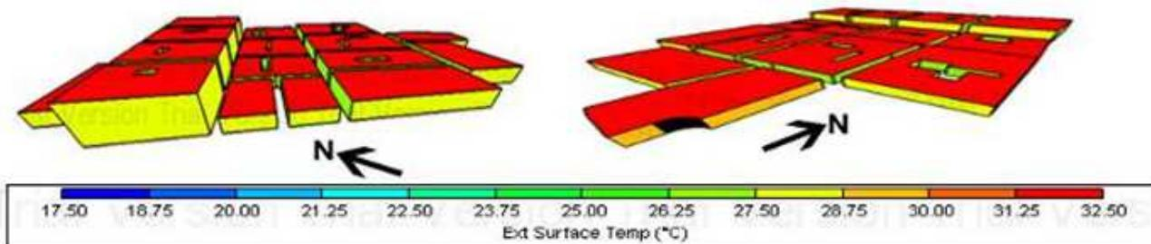
Fig. 6: Exterior surface temperature (°C) in summer. Left: Show South, West façades, right: Show North, East façades
